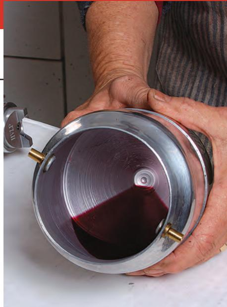
**Spit proof.** The cup from the Apollo ECO-3/E7000 system has a cone-shaped bottom, which helps keep the gun from picking up air when the fluid gets low—a helpful feature.
