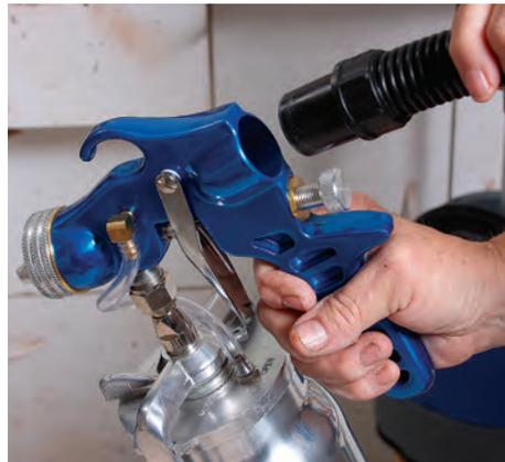
**In the way.** The hose on the Earlex SprayStation is close to the fluid-adjustment knob underneath, making it harder to turn the knob, and also to spray in tight spaces.
