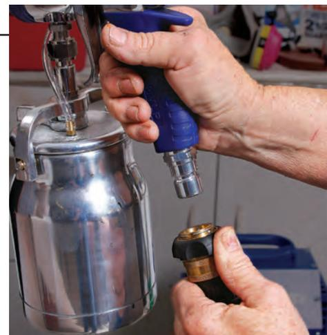
**Out of the way.** The hose on the Fuji Spray Mini-Mite 3 attaches out of the way at the end of the handle, and has an easy-to-grip coupling that makes it a snap to attach.
